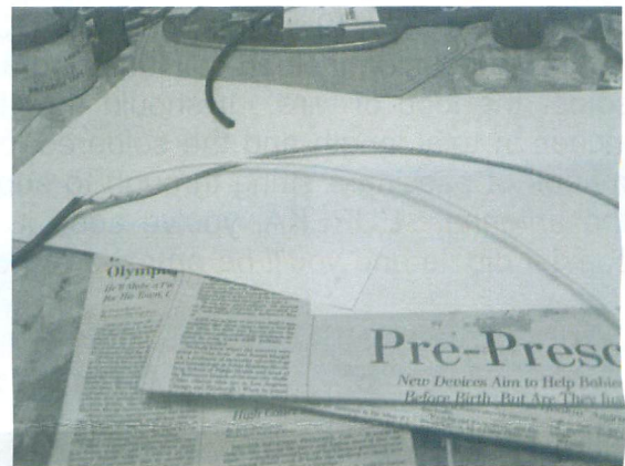
Step 8: cut away insulation
